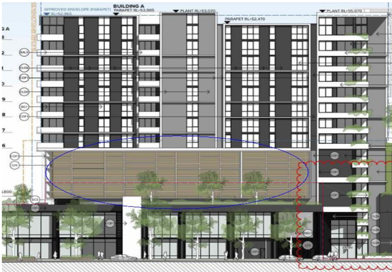
Figure 7 – Treatment of Upper Level Car Parking below Building A
